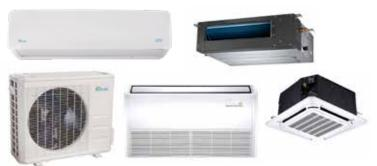
Mix and Match any Indoor Unit Style and Capacity Any style and any capacity indoor unit can be matched in a single system in any cobination, as long as the total capacity stays within the maximum and minimum allowed capacity ranges suggested for the system outdoor unit.
