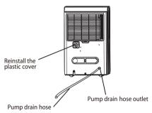
Press the pump pad of the unit to activated the pump operation. When the bucket is full the pump starts to work.
