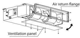
Bend the rear ventilation panel 90 degrees along the dotted line into a descending ventilation panel.(some models)
