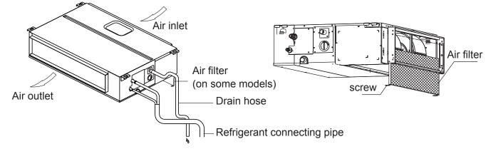
1.Put the filter into the flange subassembly through the bottom side; 2.Lock the screw.
