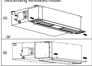
If using water, the inlet side should face down and away from the water stream.
