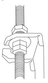
9. Mount the indoor unit onto the hanging screw bolts with a block. Position the indoor unit flat using a level indicator to prevent leaks.
